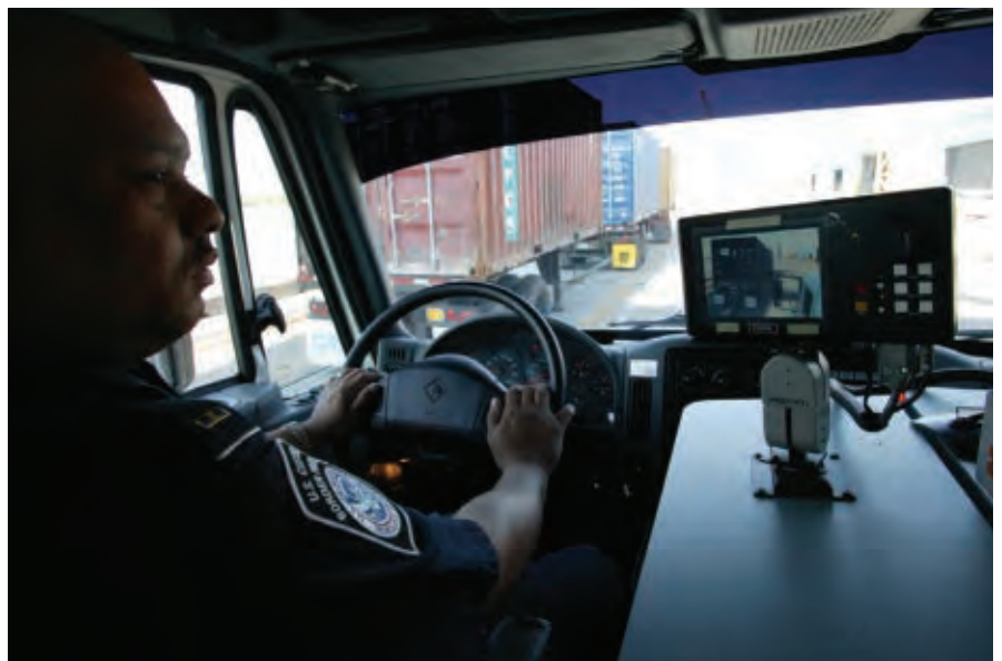
A U.S. Custom Border Protection officer watches a monitor as he operates a mobile truck x-ray over a seaport container.
