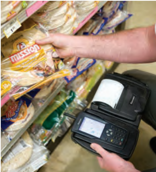
An independent distributor uses a handheld computer with attached portable printer to wirelessly transmit delivery information to Mission Foods in real time and generate invoices at a grocery retailer's store.
