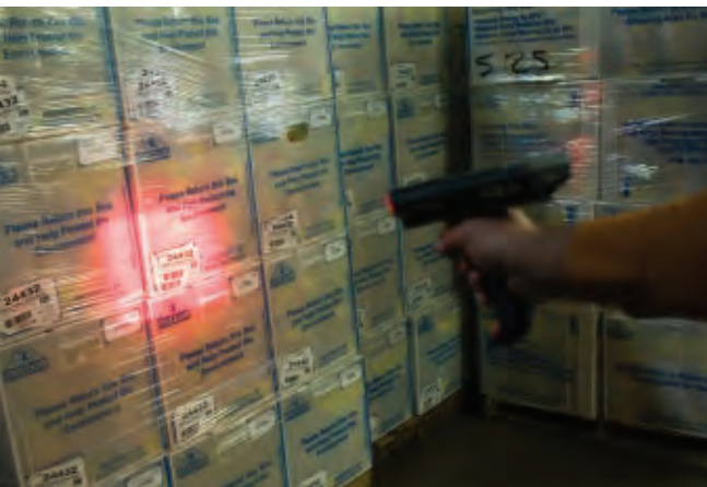
Scanning the barcode of an outbound pallet with a handheld computer equipped with a scanner and terminal emulator software.
