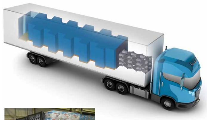
By using a "false" bulkhead at the head of its trailers, MillerCoors is able to load more cost effective and productive shipments.
