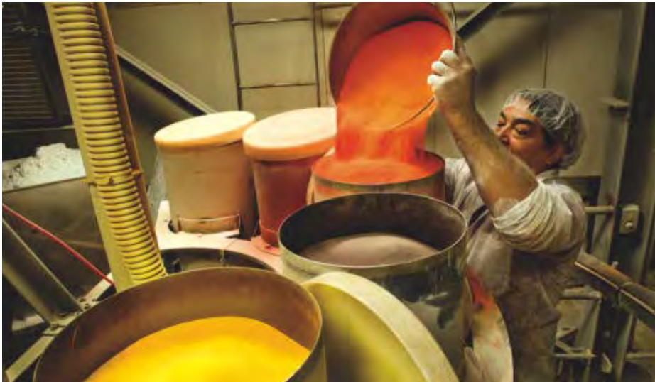
Prior to introducing raw materials into the manufacturing process (shown left), a bar code label scan captures supplier and lot information. Ce De Candy can then track that info through production (shown right).
