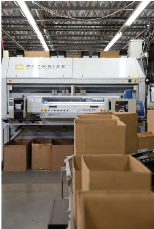
Packsizes EM7-25 machine creating right-sized boxes for induction to the picking zones.
