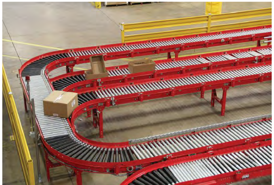
Equipment providers capture real-time information off of components, such as the rollers on a motor-driven roller conveyor, to predict when a part may fail or need maintenance.
