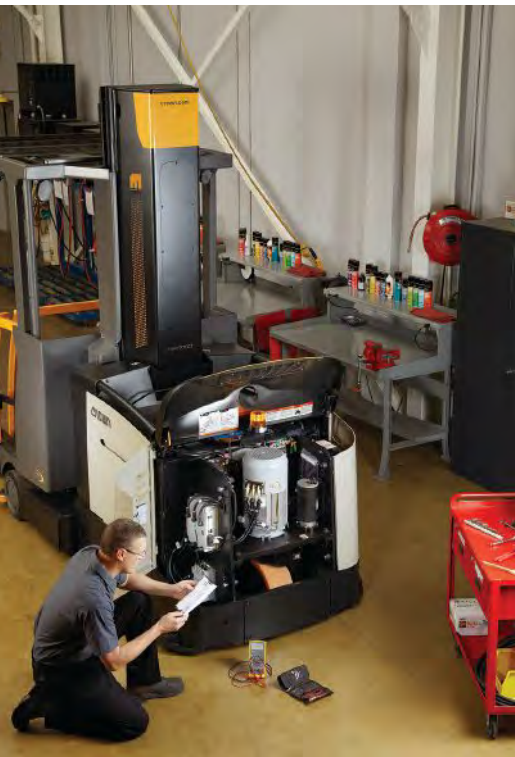
Today's lift trucks use sensors to monitor conditions on the truck and send a fault code to a technician when a component needs service.
