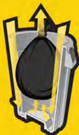
BUILT IN VENTING CHANNELS
